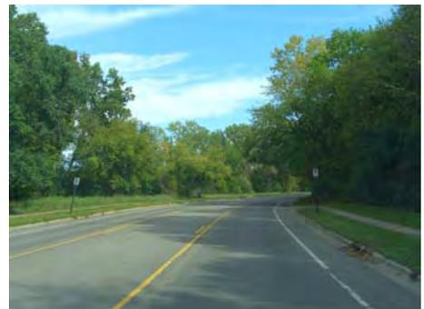
East of Kingsdale Drive on Poplar Bridge Road, the existing 3-lane 11-foot drive lane striping configuration does not provide enough space to accommodate a 6-foot bike line.
