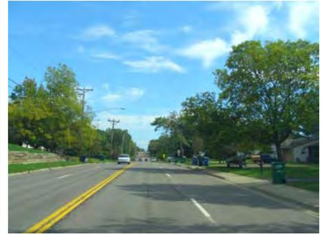
Further east on 90th Street, it would be optimal to reconfigure the 4-lane to a 3-lane layout with a bike lane. But at 44 feet wide, the bike lane would be slightly substandard, suggesting that a 2-lane approach would be more desirable if bypassing left turning vehicles onto York is acceptable.
