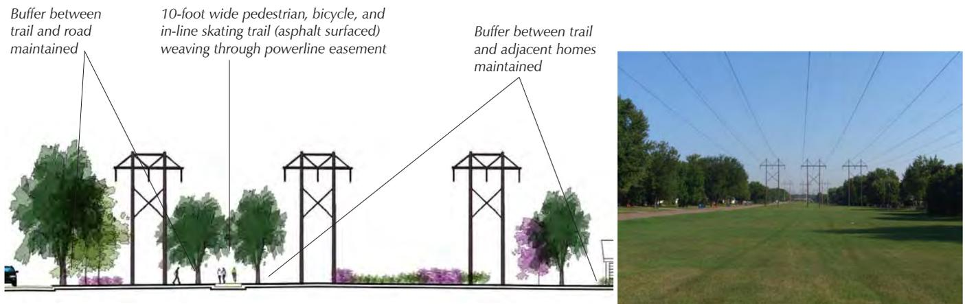
**Destination trails in Xcel Energy Corridor-type setting.** This cross-section and photo illustrate the general character of trails that follow an easement, where the objective is to maximize separation from streets and adjoining properties to enhance the recreational value of the trail.
