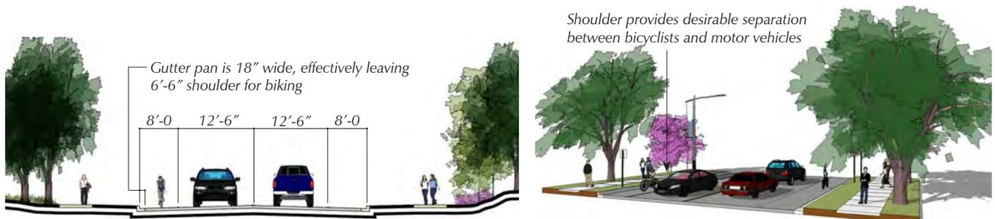
**41-Foot Street with Shoulders and Two Drive Lanes** – Under this scenario, the shoulder area on each side is held at 8 feet, allowing for two 12-foot 6-inch drive lanes. The shoulder is held at 8 feet to avoid drivers using it as a de facto drive lane. Since the shoulder area would be used for bypassing at left-turning situations, this would fall under a bike route versus bike lane designation. Compared to a 4-lane configuration, this would be a much improved situation for bicyclists.
