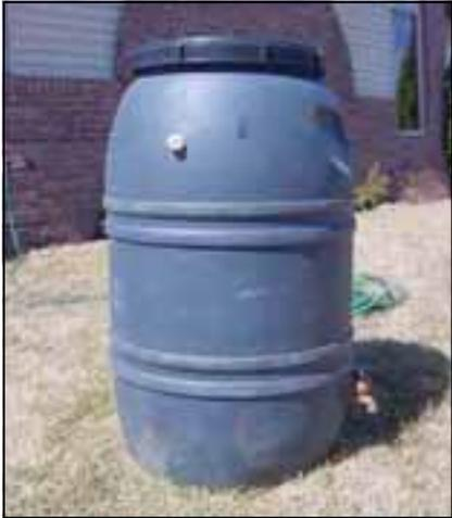
The barrel shown on the right is a typical food-grade plastic drum that you can use to build your own rain barrel. Most of these barrels are between 40 and 60 gallons and can be obtained from vendors other than the manufacturer who initially used the barrel. (See Insert 1: Local Vendors for these barrels or search the web for others.) Because of this, you will need to ask if the vendor knows the following traits for a "good" rain barrel:
