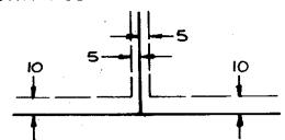
BEING 5 FEET IN WIDTH UNLESS OTHERWISE INDICATED AND ADJOINING LOT'LINES AND 10 FEET IN WIDTH AND ADJOINING STREET LINES AS SHOWN ON THIS PLAT.
