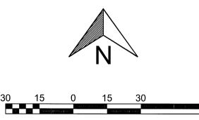
Bearings are based on the North line of Lot 3, Block 1, BLOOMINGTON 23RD ADDITION having an assumed bearing of S89°56'54"E.
