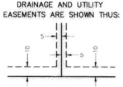
Being 5 feet in width unless otherwise indicated adjoining lot lines, and being 10 feet in width unless otherwise indicated adjoining right of way lines as shown on this plat.
