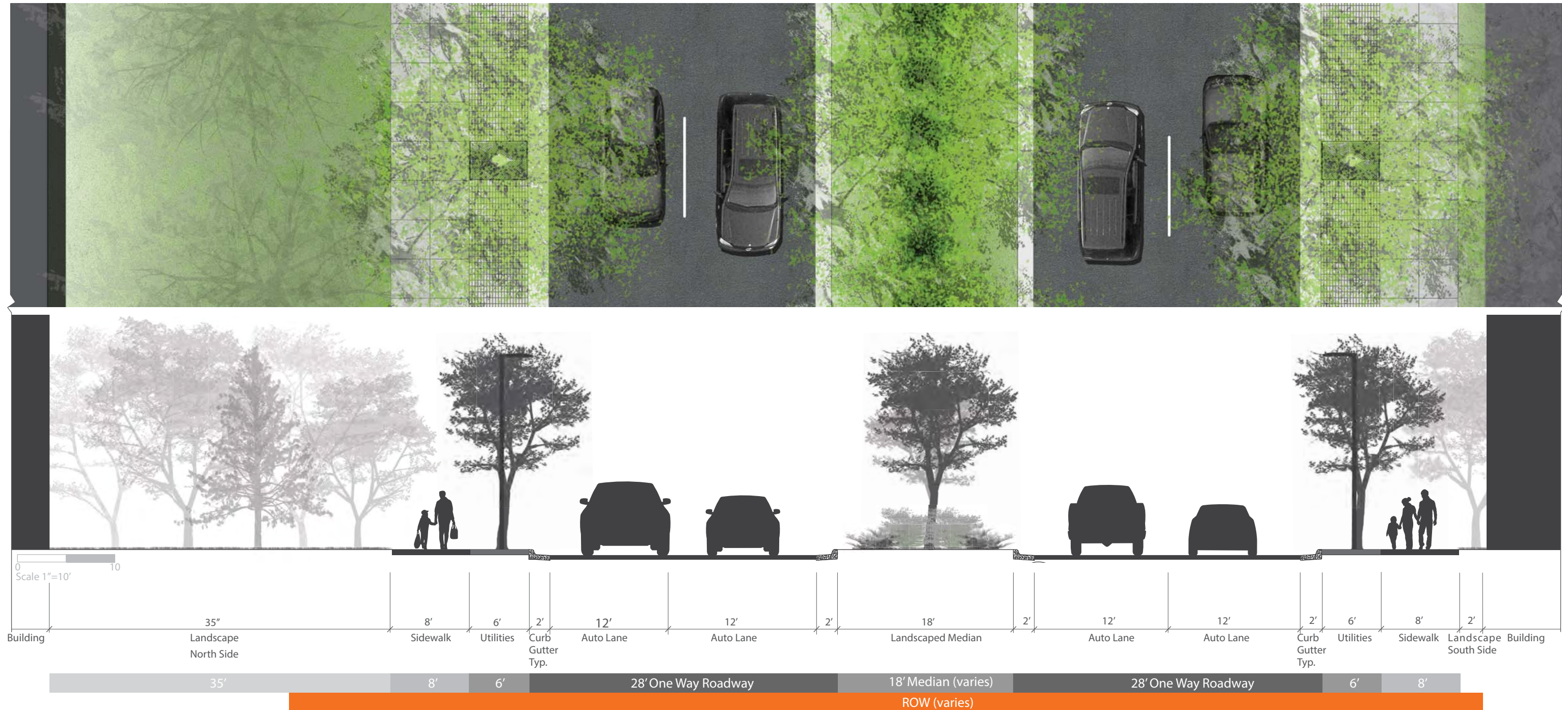
Figure 4.7 American Boulevard (East of 24th) Plan and Cross Section
