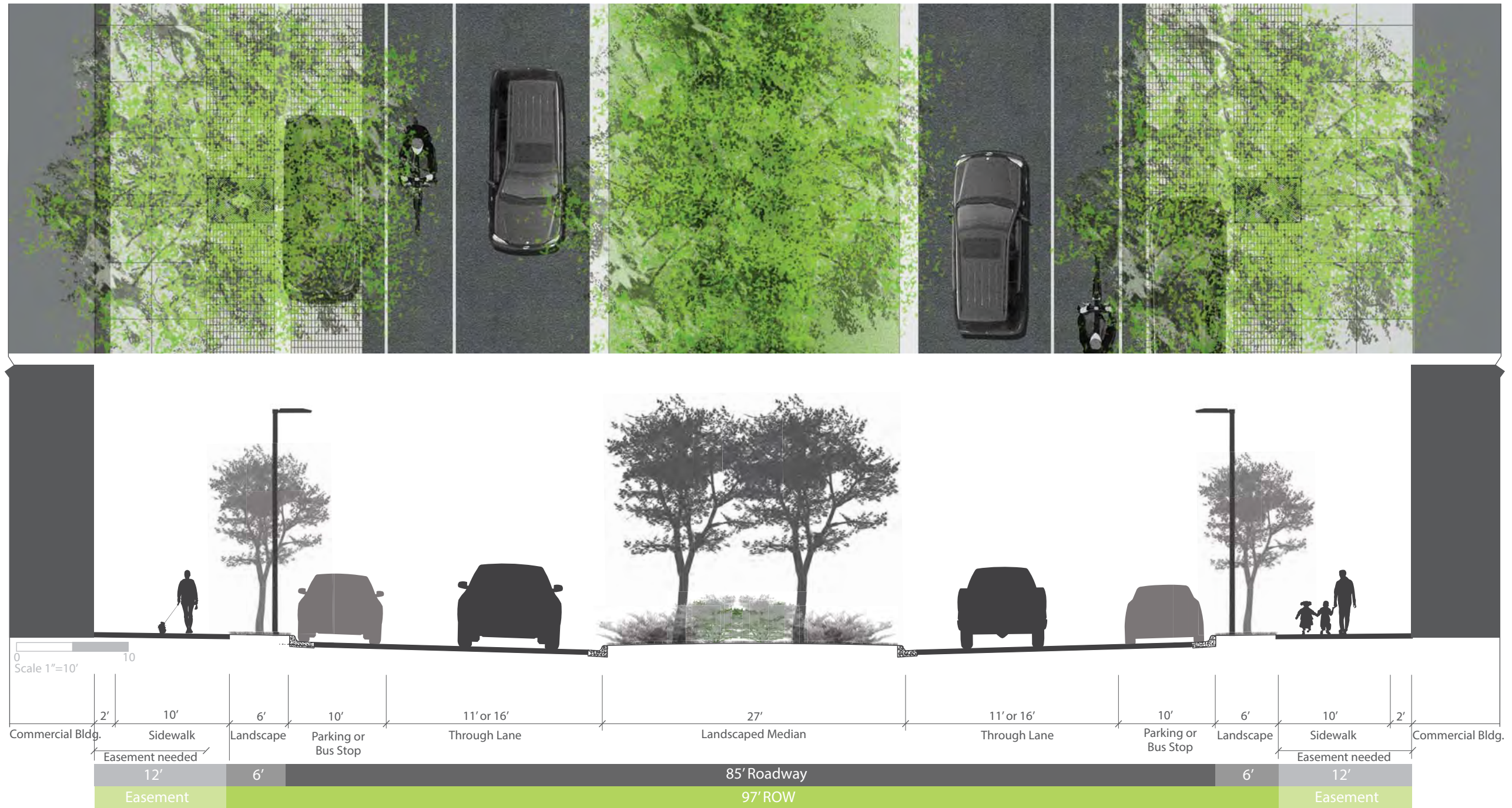
Figure 4.15 Lindau Link Proposed 2030 Plan and Cross Section
