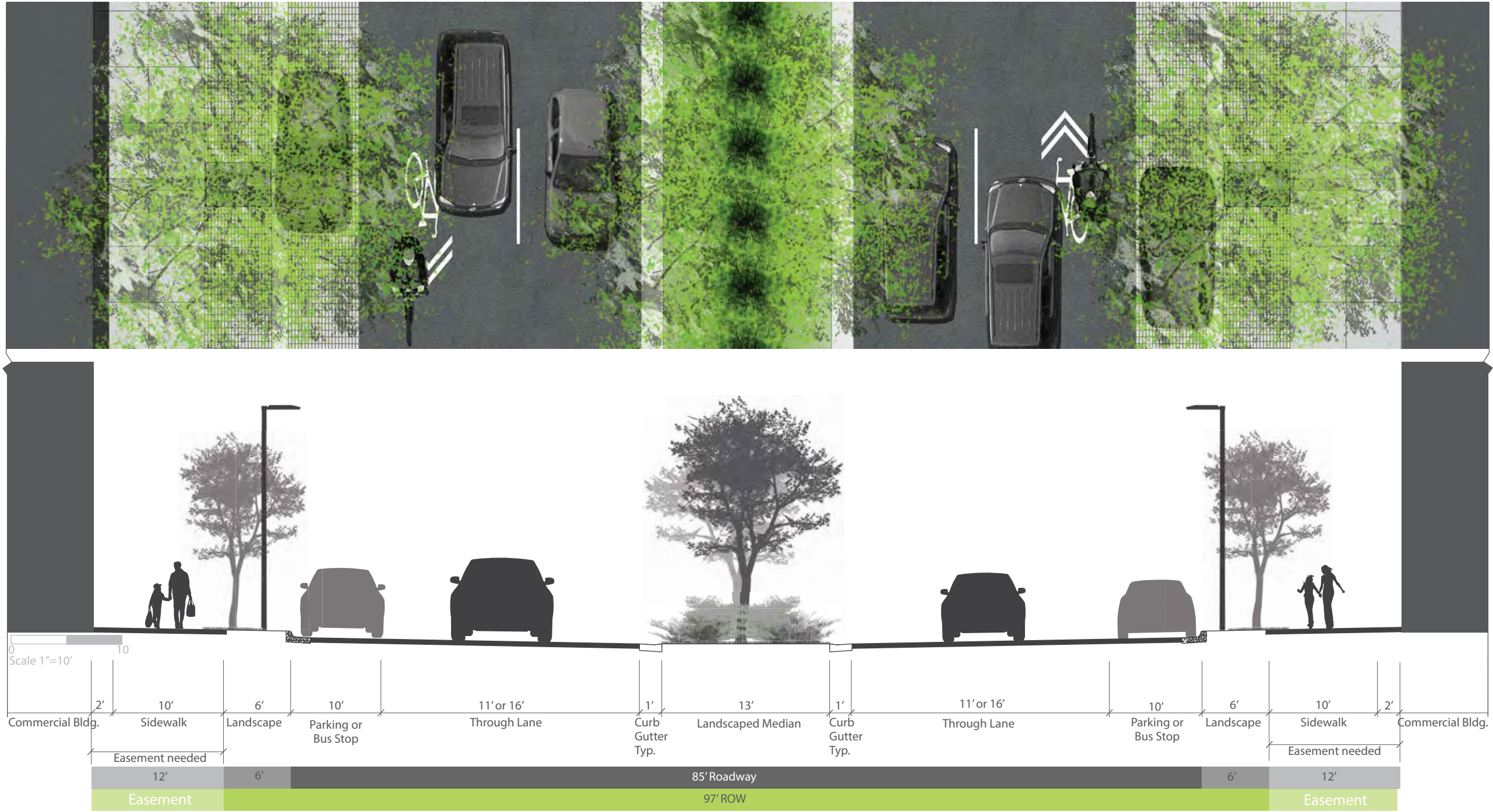
Figure 4.16 Lindau Link Proposed 200 Plan and Cross Section
