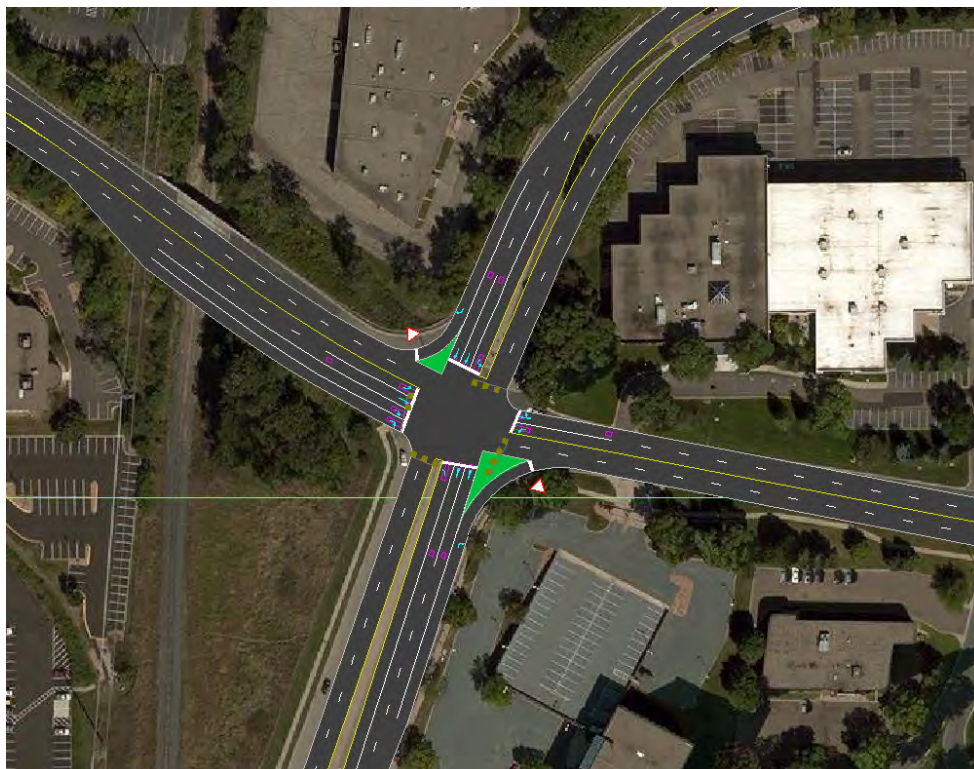
Figure 11: Long-Term Geometric Modifications to the East Bush Lake Road/78th Street Intersection
