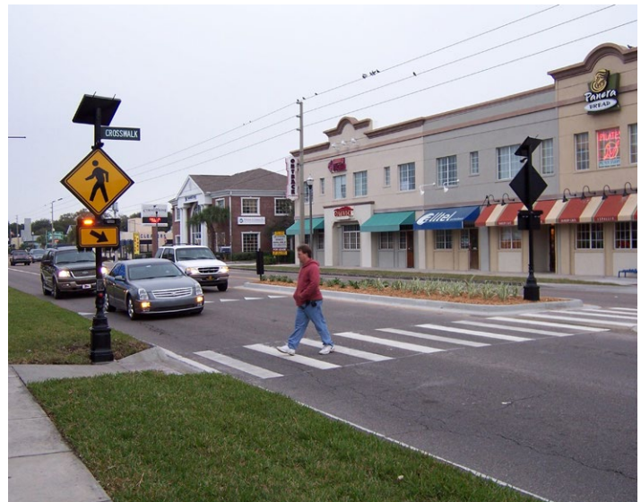
Mid-block crossing with pedestrian activated flashing lights and median island
