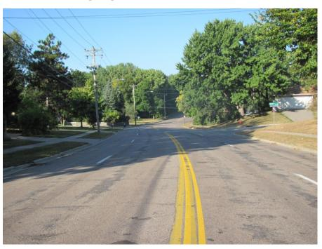
The intersection of 84th Street/Xerxes Avenue is a T-intersection currently controlled by an old span wire traffic signal that has reached the end of its service life and is due for replacement. In addition to the age of the traffic signal, steep grades west of the intersection create sight distance issues for motorists waiting on the south approach of Xerxes Avenue to enter 84th Street.
