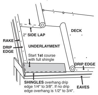
**Installation:** When applying underlayment, keep the product as wrinkle-free as possible. Unroll the underlayment parallel with the eaves. When drip edge flashing is installed, the underlayment should go over eaves' drip edge flashing, but go under the rake's drip edge flashing.
