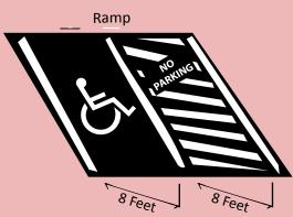
Access aisle needs to be located on Ithe passenger side of the space.
