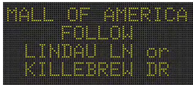
Figure 4: Overhead Dynamic Message Sign
