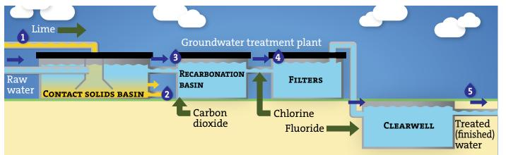
The softening process begins when slaked quicklime is mixed with raw water in one of the City's two solids contact basins. Each basin holds 550,000 gallons of water.
