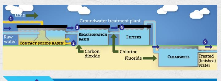
The softening process begins when slaked quicklime is mixed with raw water in one of the City's two solids contact basins. Each basin holds 550,000 gallons of water.
