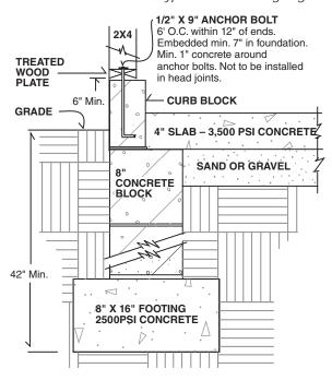
**Note:** Anchor bolts are a maximum of 6' O.C., 12" within any end or splice and minimum two per board.
