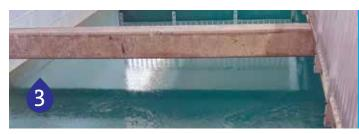
The water enters a recarbonation basin where it is adjusted to the proper pH by adding carbon dioxide. A precise amount of chlorine is added to discourage bacterial growth as the water travels through the City's distribution system.
