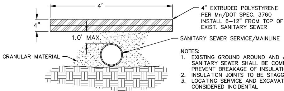
**411 - SANITARY SEWER INSULATION DETAIL**
