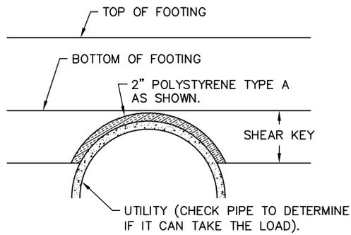
**129 - PIPE UNDER SPREAD FOOT. (THUR SHEAR KEY)**
