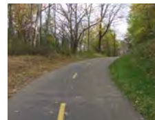
A broken solid yellow line is used on busier trails to remind trail users to stay in their lane. Consistency of use along a trail is important in order for trail users to understand the pattern.
