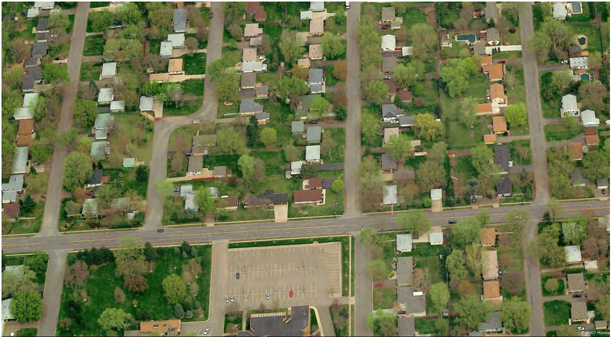
Aerial image of the eastern side of the city illustrates that sidewalks are primarily provided along major streets and not along local streets in the neighborhood. Through education and enforcement, drivers of motor vehicles need to be reminded that local streets are inherently multi-modal, with pedestrians, bicyclists, and motor vehicles all sharing the same space. Incidentally, in Bloomington, the accident rate between motorists and pedestrians in these neighborhoods is quite low.
